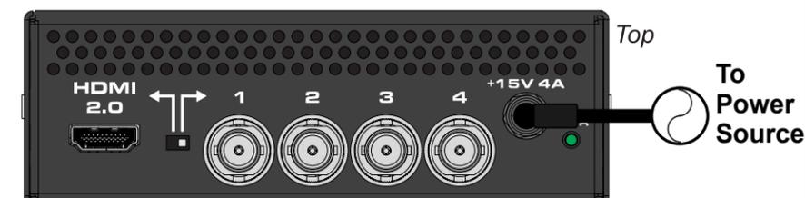
**Note:** The NEWT-IPX powers on automatically when the power supply is plugged in.
